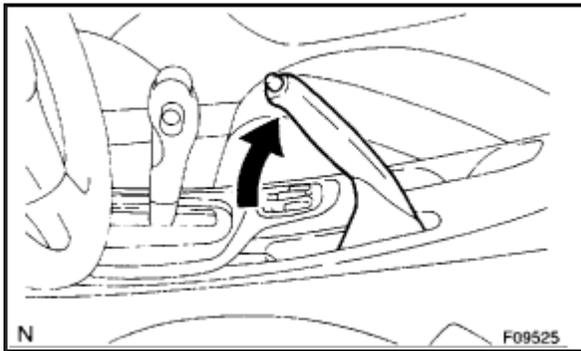
1. CHECK PARKING BRAKE LEVER TRAVEL Pull the parking brake lever all the way up, and count the number of clicks. Parking brake lever travel at **196 N (20 kgf, 44.1 lbs)** : **5 - 8 clicks** If incorrect, adjust the [parking brake](#).
