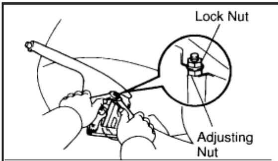
2. IF NECESSARY, ADJUST [PARKING BRAKE](#) **HINT:** Before adjusting the [parking brake](#), make sure that the rear [brake shoe](#) clearance has been adjusted.
