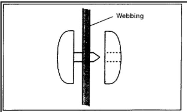
**HINT:** Press the adjustment screw in order to position the male and female parts of the Tongue Plate Stopper parallel to each other, as shown in illustration.
