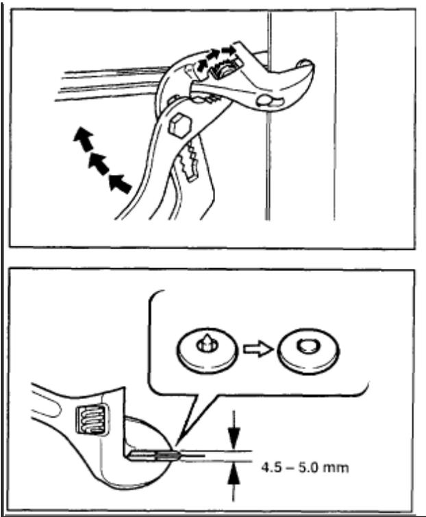
C. When the adjustment screw for the adjustable wrench can't be turned by hand, tighten the adjustment screw using a pair of adjustable joint pliers until the space between jaws of the adjustable wrench is 4.5 - 5.0 mm. (See illustrations.)
