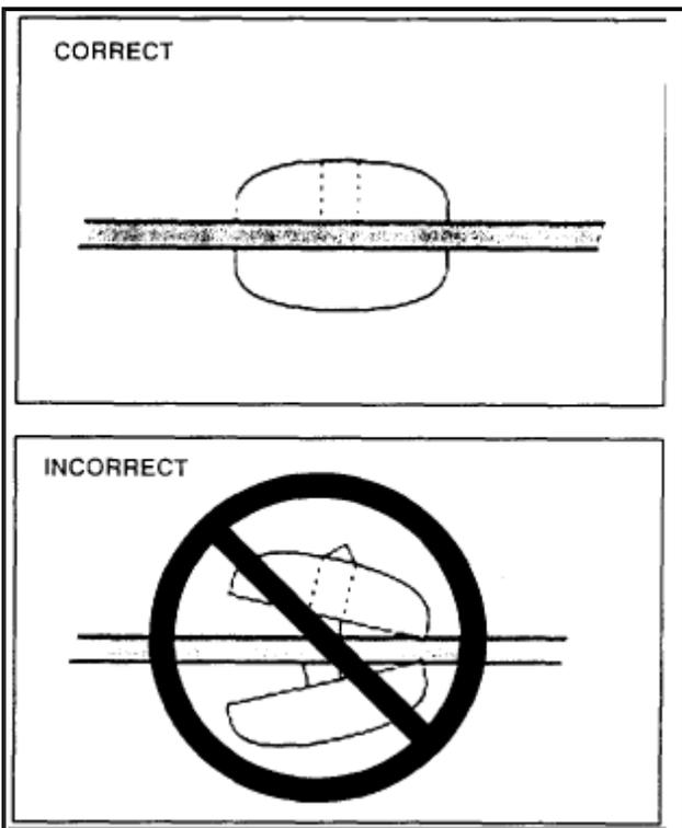
D. Check to be sure that the male pin of the Tongue Plate Stopper has become deformed evenly in the hole of the female part and is firmly held to the belt webbing. (See illustrations.)
