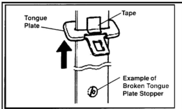
A. Shift the Tongue Plate to the upper portion of the Tongue Plate Stopper, and temporarily hold it with a clip or tape.
