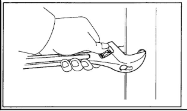
B. Pinch the Tongue Plate Stopper into the webbing using an adjustable wrench, and turn and push the adjustment screw by hand.
